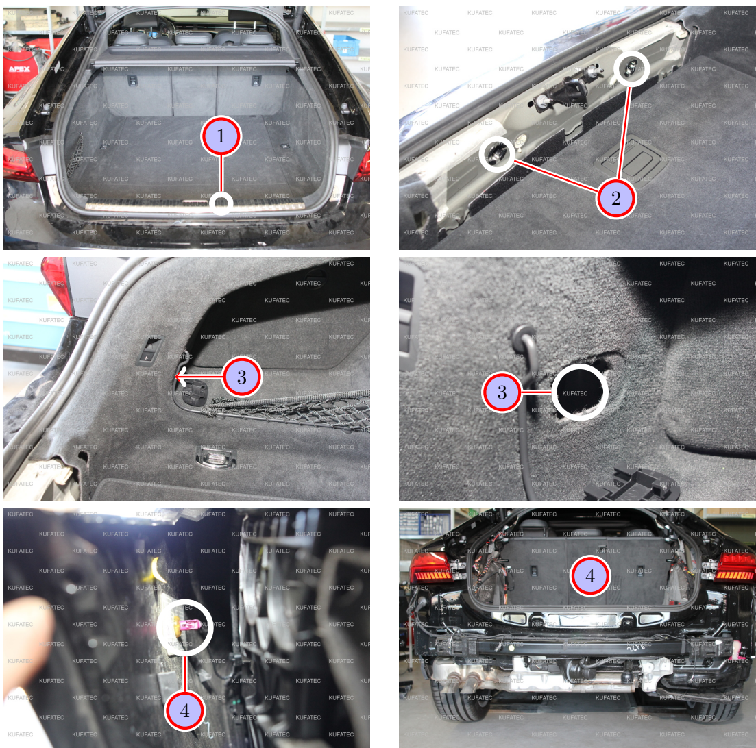
Figure 9: Disassembly rear bumper
